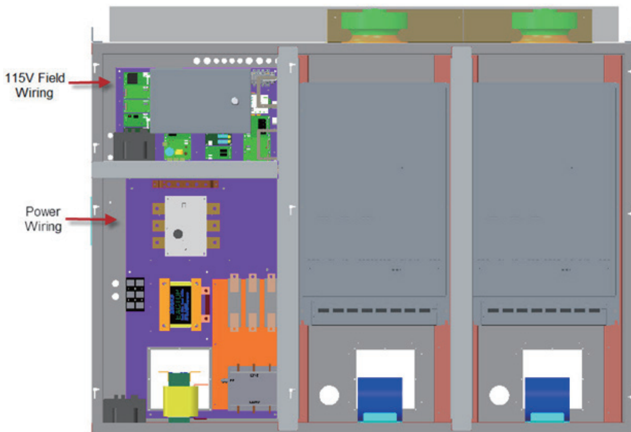
Figure 25. Power Entrance of AFD panel
